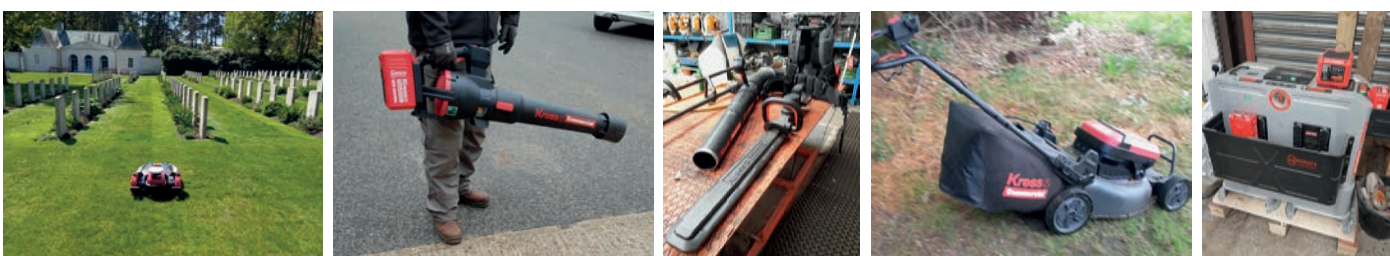
Trialling a suite of electrical machinery at Brookwood Military Cemetery (UK) (left to right): a robotic mower, a leaf blower, a hedge trimmer, a rotary mower & a portable power bank charger.
